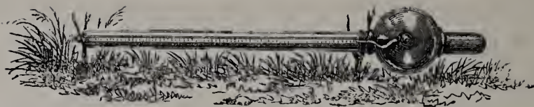
FIG. 116.—Solar radiation thermometer. Blackened bulb in vacuo.
